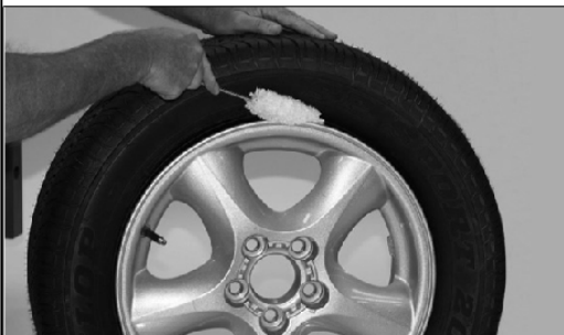
Figure 5 - Apply Rubber Lubricant to Tire Beads
