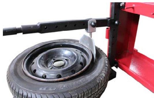
Figure 3 - Position Tire and Bead breaker shovel
