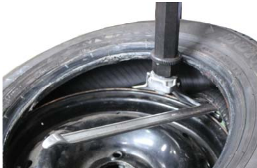
Figure 13 - Guide Lower Bead Over STL and Over the mounting head
