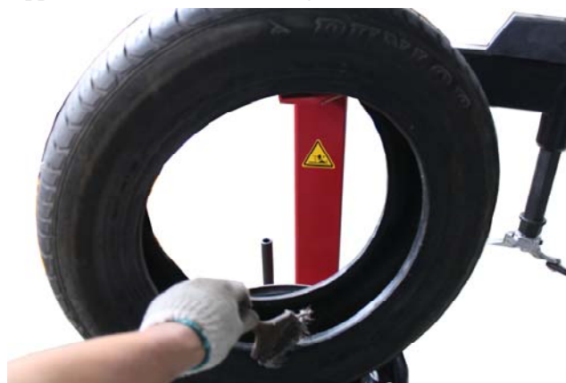
Figure 16 - Lubricate Tire Beads Liberally
