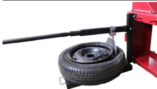
Figure 3 - Position Tire and Bead breaker shovel
