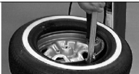
Figure 12 - Demounting Lower Bead
