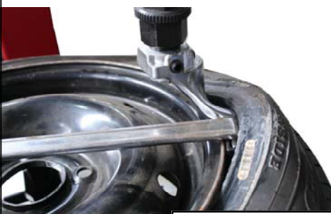
Figure 11 - Lift Bead Over Demount Head
