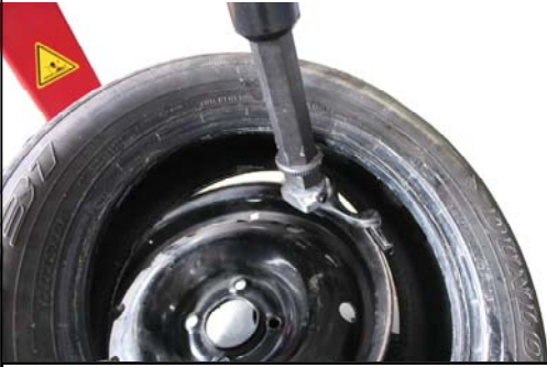
Figure 17 - Position Tire Against (Mount/Demount Tool)
