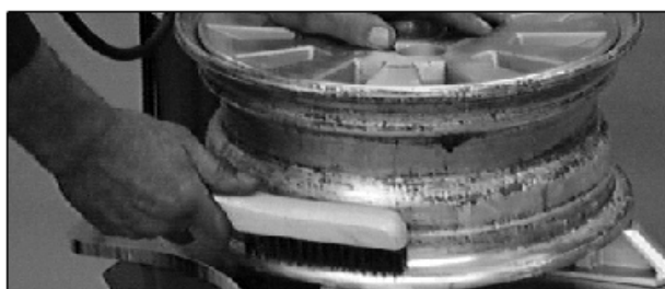
Figure 15 - Inspect and Clean the Wheel
