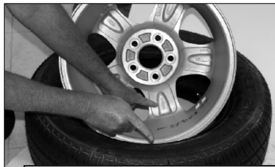
Figure 14 - Verify Size Match Between Tire and Wheel
