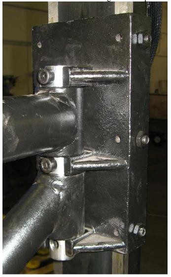
15. Now use up/down switch to raise preinstalled rod up and inside RAA-002 as shown below. Then use the other RAA-008 mounting bolt to finish connection.
