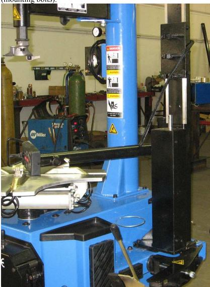
10. Place RAA-001 mounting plate on main machine body and align with the holes. Use some tape to hold RAA-001 plate in place. Position RAA-011 main assist arm in position as shown in above picture. Use RAA-007 mounting bolts to bolt RAA-011 and RAA-001 to main machine body. RAA-001 mounting plate must be placed under RAA-011. This allows the bead breaker arm to move freely under without rubbing on RAA-011.
