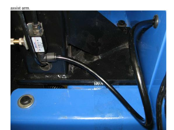
12. Connect air to the air gauge on back of machine. Use your own regulator on your
