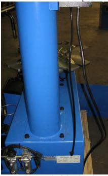
6. Open side panel of the tire changer. Install the two size 10 hoses to the bottom of the large vertical main column. These 2 air lines are identical and can be
