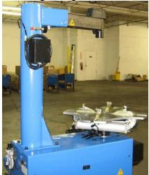
3. Place hexagon mounting bar through hole in horizontal swivel bar. The place the large spring over the hexagon bar. Next with the help of another person, push spring down while placing plastic cap on top of hexagon bar and use the hex bolt
