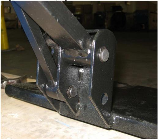
9. Assist arm assembly begins by mounting RAA-011 (main assist arm column) to main side of tire changer body using RAA-001 (mounting plate) RAA-007
