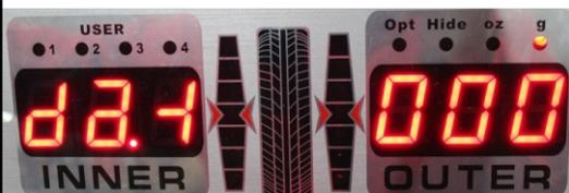
Press B+ or B – to adjust diameter measurement. (1 unit = 0.1 inch).
