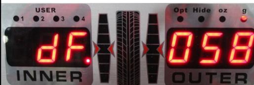
Press B+ or B – to adjust the DF value of offset error.
