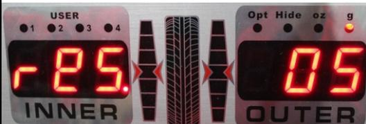
Press B+ or B – to adjust the RES value of Residual value of showing
