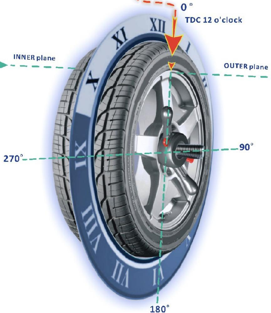
**Step 3 :**
