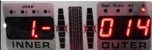
Press B+ or B – to adjust the I value of axial error.
