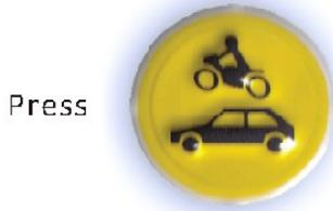
Vehicle MODE Key to enter the motorcycle wheel balancing mode.
