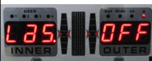
Press B+ or B – to adjust laser pointer on or off.
