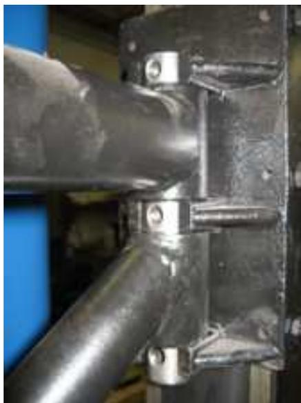
6. Then use 2 of RAA-008 mounting bolts in top 2 holes of RAA-002.
