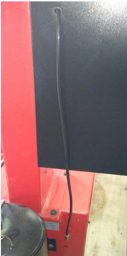
5. Install swing arm tower on machine using 4 bolts X95-16. Feed hose through hole on body of machine while mounting tower. Caution! The powder coating is very slick. You should have 2 people to assist with this process in order to not cause injury or damage to yourself or the machine.
