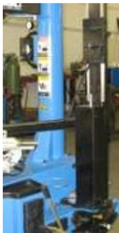
2. Position RAA-011 main assist arm in position as shown in above picture. Use RAA-007 mounting bolts to bolt RAA-011 to main machine body.
