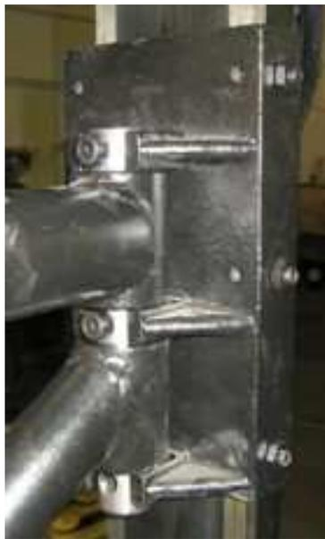
7. Now use up/down switch to raise preinstalled rod up and inside RAA-002 as shown below. Then use the other RAA-008 mounting bolt to finish connection.
