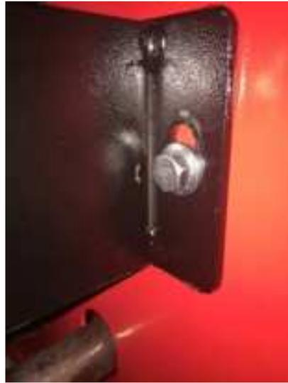
10. Install air distributor on air tank as shown in picture. Two large lines route from top of air distributor directly out top on machine to turn table. Single line routes from bottom of air distributor to inflation pedal valve.
