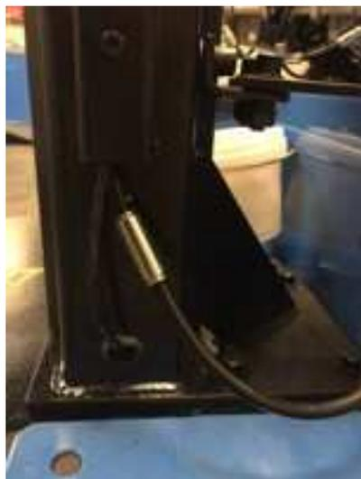
4. Follow hose from oiler inside machine and splice hose. Use T fitting that was provided and connect hose from assist arm inside machine.
