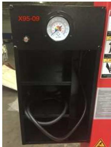
9. Install air tank using 2 bolts. Ensure air tank is positioned as high as possible before tightening bolts. See below pictures.
